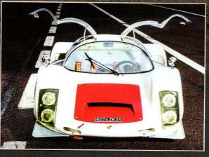
Gullwing doors were necessitated by the shape of the roof - it would have been impossible to use conventional doors with such a curved roof and wide sills. The Cd figure was 0.35 - slightly higher than the outgoing 904...
